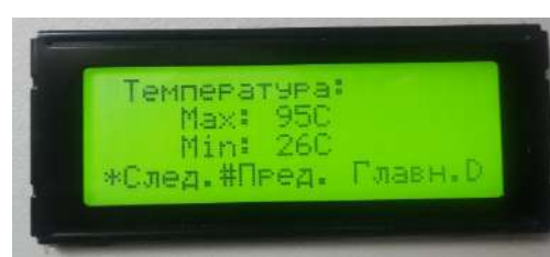
f) The menu for setting the maximum and minimum temperature values
