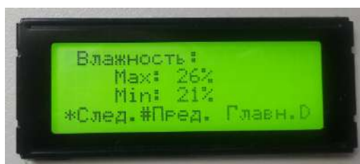
e) The menu for setting the maximum and minimum humidity values
